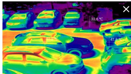
Parking lot with the temperature measurement
